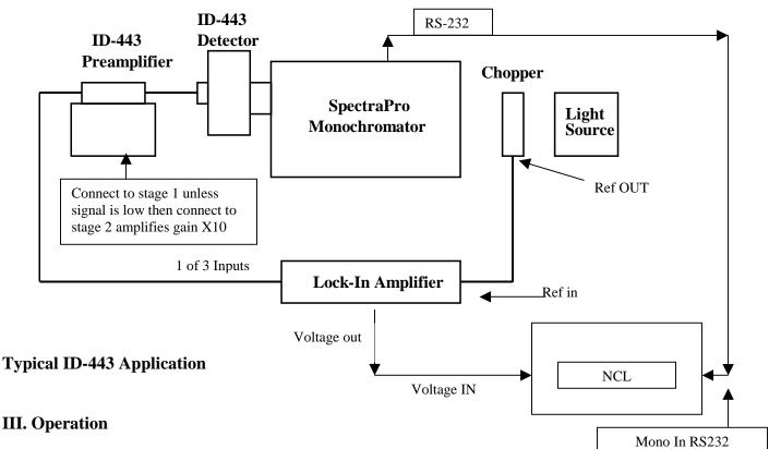
Refer to the instructions provided by Manufacturer on the detector and preamplifier before switching on the power to the preamplifier. The detector must be cooled with liquid nitrogen before operation.
