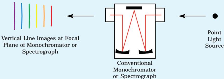
**Figure 7: Collecting Multiple Spectra Simultaneously**
