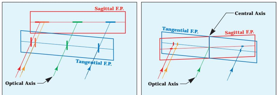
Tangential and sagittal focal planes are formed by the use of spherical mirrors at off-axis angles. A detector on the tangential focal plane detects sharp vertical lines for best spectral resolution.
