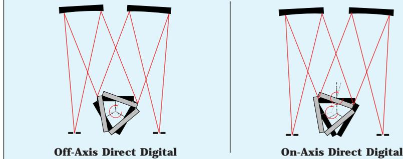
**Left: Off-Axis Grating Rotation:** Multiple gratings are mounted on a turret which rotates about its central axis. ARC's optical system is set up to fully illuminate each grating throughout its entire scanning range, thus throughput is maximized. This simple and rugged drive arrangement allows for both wavelength scanning and grating changes with a single motor/gear arrangement.
