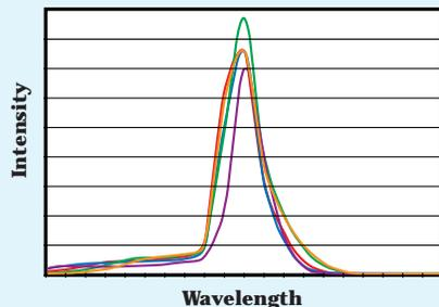
Spectral resolution varied from 0.13nm to 0.17nm fwhm across a 25mm wide focal plane for the on-axis instrument. This is a total variation of 0.04nm.
