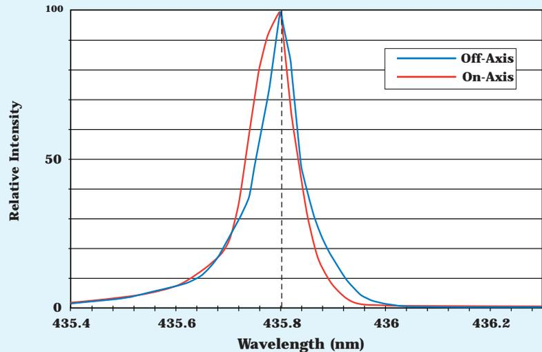
**Figure 4: Spectra lines produced by on-axis and off-axis scanning monochromators**
