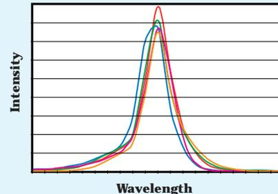
Spectral resolution varied from 0.15m to 0.16m across a 25mm wide focal plane for the off-axis instrument, for a total variation of 0.01nm.
