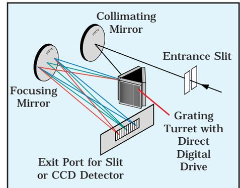
Figure 1: Spectrometer Optical System
