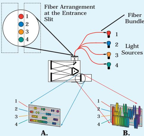
A four leg fiber bundle collects light from four different sources to the spectrograph and CCD detector.
