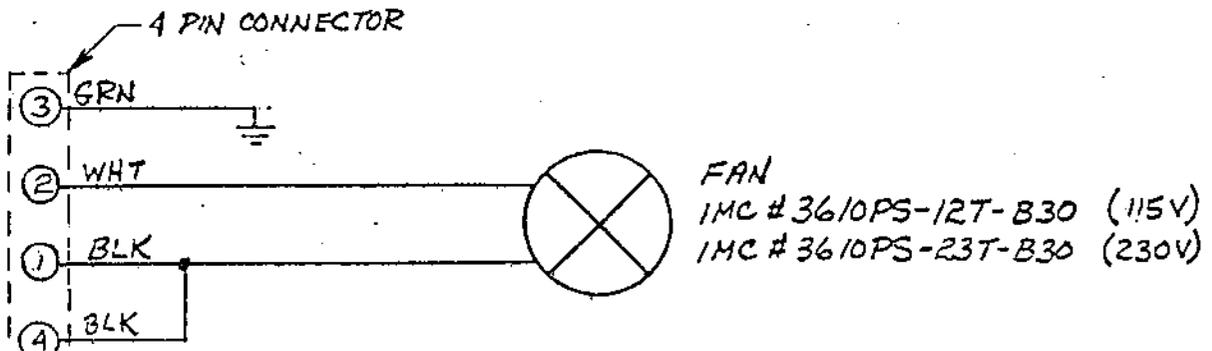
6. USE 20 AWG STRANDED WIRE FOR CONNECTIONS TO  $\frac{1}{16}$  & FAN
