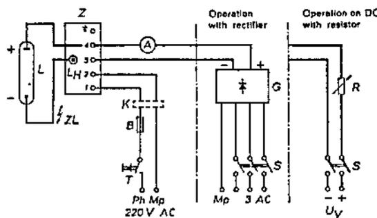
Fig. 1: XBO lamps with or without ignition electrode.
