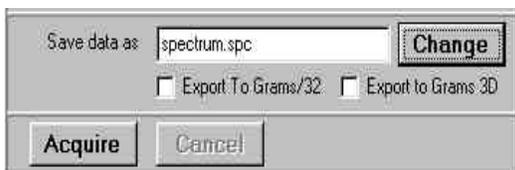
In the Acquisition screen, if you specify a filename using the SPC format in the Save dialog box, two check boxes will appear. They are Export to Grams and Export to Grams 3D. If one of these boxes is checked, the data will be passed to the program and will appear in the working window. This method has the advantage, when taking
