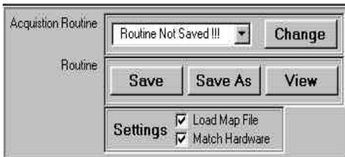
The Routine panel is used to recall or create new acquisition routines. The choice box will display “Routine Note Saved!!!” if the current conditions have not been recalled from a stored routine file. The most recently used stored routines are shown as choices in the panel. If the desired routine is not displayed here, clicking on the Change button will allow you to browse through your directories and recall the desired routine.
