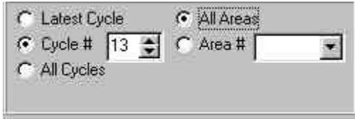
When acquiring spectra it is possible to display the data in different ways. If there were multiple cycles specified in the acquisition it is possible to view at any time, the latest cycle (spectrum) acquired, or the Nth previous cycle (spectrum) individually or all of the currently acquired cycles.
