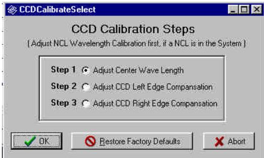
The introductory screen for the calibration procedure will be displayed. Note that you will repeat the procedure three times to accurately calibrate your system. Start out by selecting Step 1 and then click on the OK button. If at any time you feel that you made an error you can always click on the Restore Factory Defaults button.
