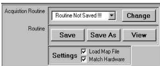
The Routine panel is used to recall or create new acquisition routines. The choice box will display “Routine Note Saved!!!” if the current conditions have not been recalled from a stored routine file. The most recently used stored routines are shown as choices in the panel. If the desired routine is not displayed here, clicking on the Change button will allow you to browse through your directories and recall the desired routine.
