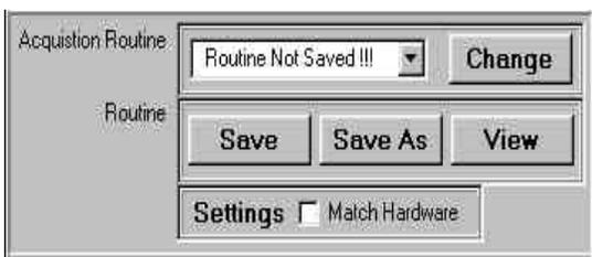
The Routine panel is used to recall or create new acquisition routines. The choice box will display “Routine Note Saved!!!” if the current conditions have not been recalled from a stored routine file. The most recently used stored routines are shown as choices in the choice field. If the desired routine is not displayed here, clicking on the Change button will allow you to browse through your directories and recall the desired routine.
