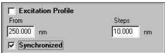
If neither the Excitation Profile nor Synchronized boxes are checked, the monochromator will move to the specified wavelength and stay there through all of the spectral acquisitions specified in the panels above.
