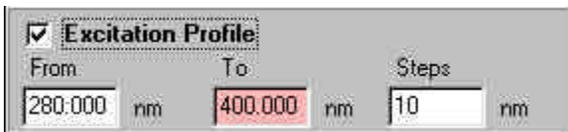
The Excitation Profile panel will appear if your system includes two spectrometers and you are using one in conjunction with a light source for fluorescence excitation. If the check box is not
