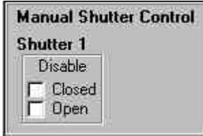
If a CCD is in the current light path, the CCD manual shutter control panel will appear. The shutter is normally closed, opening only for the specified integration time. By clicking on either of the options boxes here, you can keep the shutter permanently open or permanently closed.
