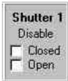
The Shutter control panel allows you to disable the mechanical shutter opened or closed for subsequent read outs. For experiments where spatial information in the vertical direction is not important, and read out speed is, it may be advantageous to disable the shutter in the open position.
