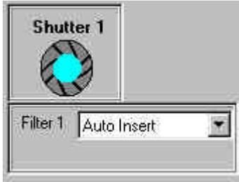
If your system has an automated shutter its current status, i.e. open or closed is shown in the shutter panel. Click on the shutter icon to change the state of the shutter. If an automated filter wheel is present, the Filter panel will appear. The choice field shows the current filter in place or Auto Insert if this option has been defined in the Hardware Configuration. You can insert any filter by clicking on the choice arrow and highlighting the appropriate filter.
