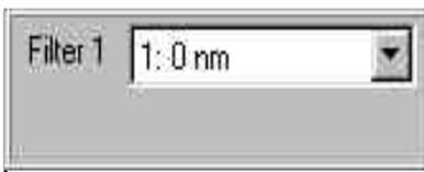
The filter panel appears if there is a filter wheel in your current experimental setup. The field shows the current filter position, or cut off wavelength, if specified, or name specified in the filter wheel set up tab in the hardware configuration screen. Click on the arrow to display all possible choices and highlight the desired filter.
