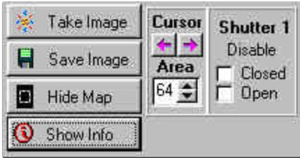
The options available for the lower window when in spectral mode include: Take Image where in a new image is taken and displayed in this window. Save Image will save the current image in the window to a BMP, Tiff or SPC file. Hide/Show Map will trace the current map on the image in the window. The Show/Hide Info button will toggle between the information screen shown above and the last image taken. The Area and cursor arrows will show the intensity and wavelength values for
