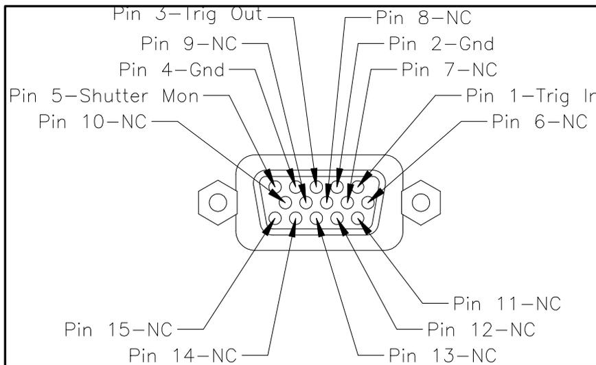
***InSpectrum* Trigger connector pin assignments**
