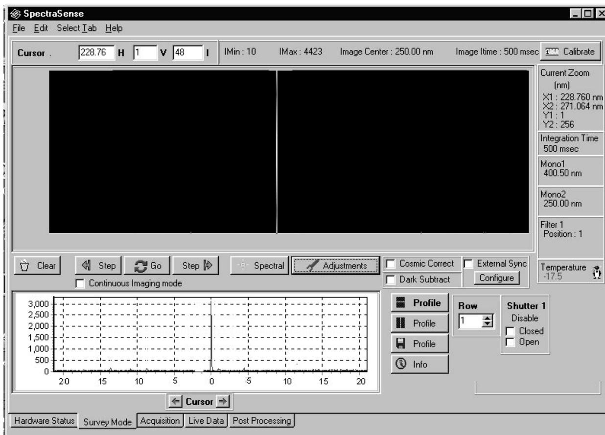
If your instrument passed step one, but failed step 2, it is highly probable that light is not entering the spectrograph. Perform the diagnostics in part 2 of the troubleshooting section.
