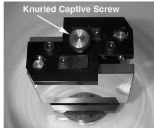
To remove the turret from the container, apply a slight downward pressure on the top of the turret and unscrew the knurled captive screw. Lift the turret out of the container by the capture screw being very careful so as to not allow the face of the grating to touch the wall of the container. To store the turret follow the reverse procedure.
