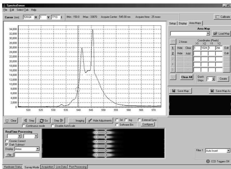
You should now see two spectra on the screen. Their intensities may not be equal, however the peak positions should be the same. If there is a greater than 2 pixel shift in the positions of the peaks, perform the same procedure with the other grating on the turret. If the peaks superimpose with one grating and not the other follow the procedure
