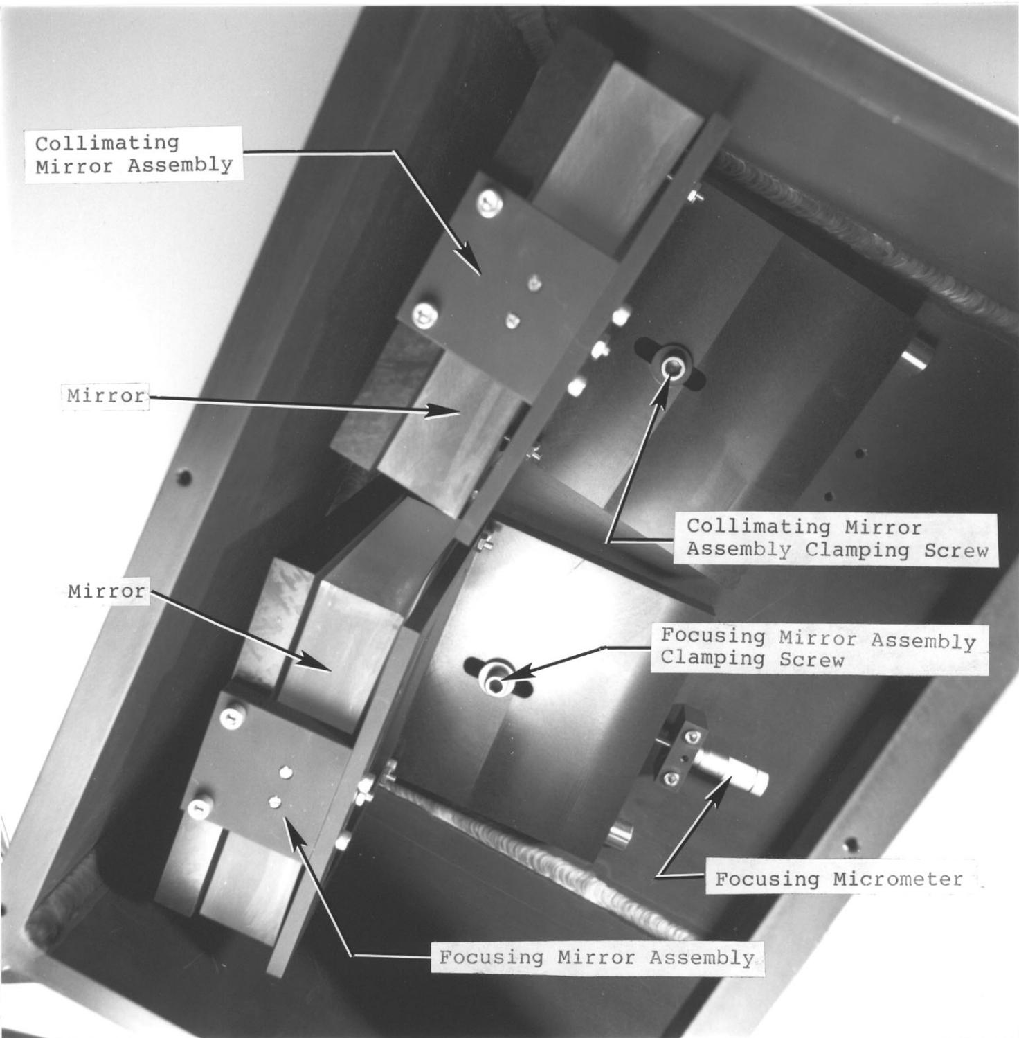
**FIGURE 4: GRATING ASSEMBLY IN PROTECTIVE SHIPPING/STORAGE BOX**
