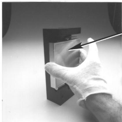
Grating is Tilted Back Toward the Grating Holder until the Half Ball Locates in the Spring Hole
