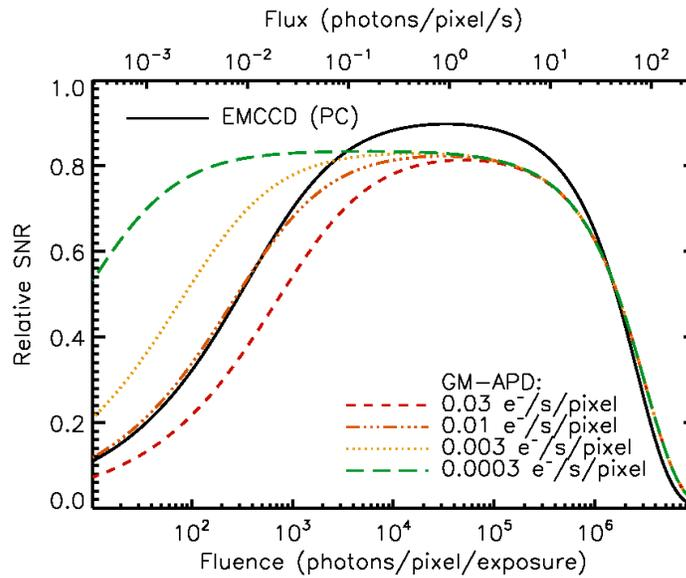
Figure 9. This plot shows relative SNR (normalized to  $\sqrt{\text{Fluence}}$ ) for a state-of-the-art EMCCD and GM-APDs with various values for dark count rate. The current state-of-the-art DCR for the GM-APD is shown, as well as 1/3, 1/10, and 1/100 reduction in DCR. For even the 1/3 reduction in DCR, the GM-APD is comparable to EMCCD performance due to the clock-induced-charge that plagues the EMCCD.
