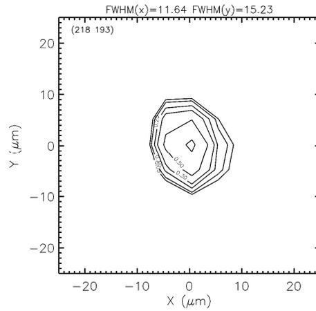
*Figure 8. This plot shows the intra-pixel sensitivity of a single pixel. The response is normalized to the peak response of the pixel. This measurement shows that the pixel response drops sharply away from the pixel center.*
