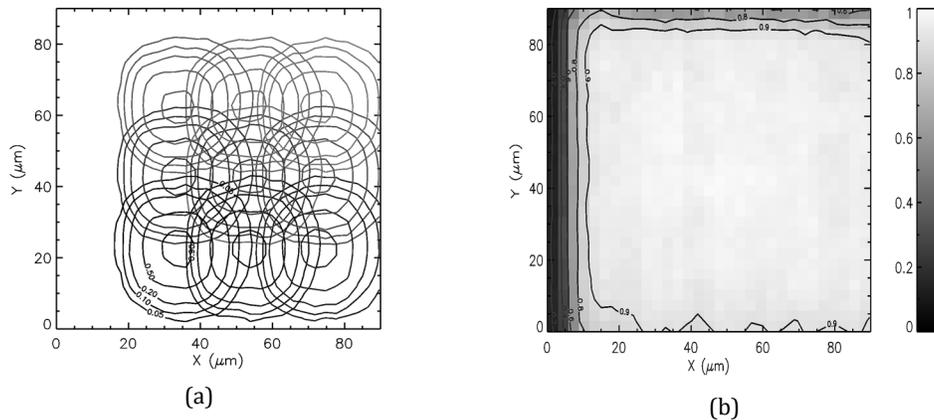
*Figure 3. These plots show the intrapixel sensitivity of the 9A. A raster scan with  $2 \mu\text{m}$  spacing was done on a region covering  $3 \times 3$  pixels using a circular beam ( $7 \mu\text{m}$  FWHM). The contour plots show the responses of the nine pixels overlaid on the same plot (a). The signal from each pixel is summed at each location of the beam and plotted, showing the summed response is uniform throughout the entire  $3 \times 3$  pixel region (b).*
