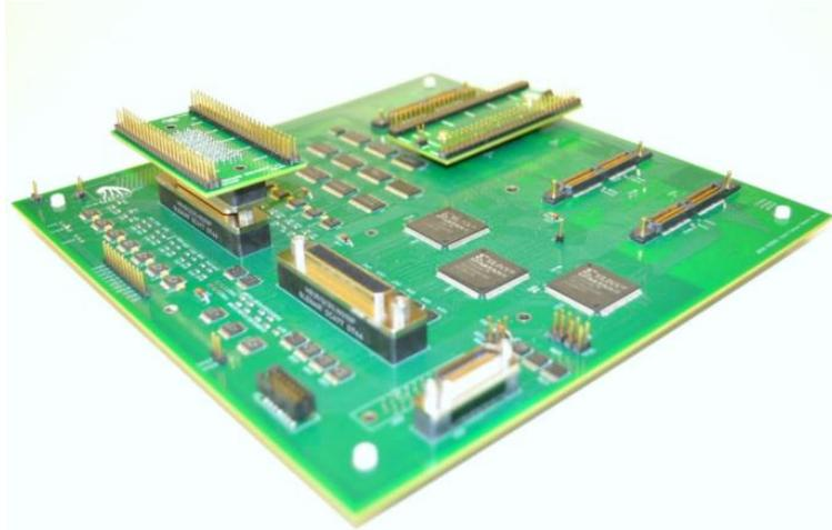
*Figure 25. This image shows a cryogenic multi-layer circuit board designed in the CfD and populated in CEMA. All of the components on this board will be exposed to temperatures as low as 40 K, nanoTorr pressure levels, and high energy particle radiation.*
