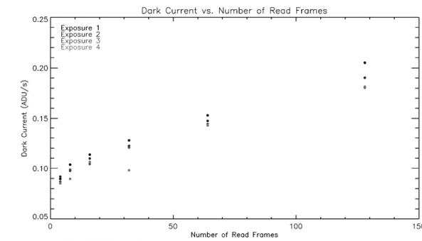
Figure 12. This figure shows the measured dark current of a detector, measured using the JMCE control electronics, in an experiment run by Joseph to examine dark current versus the number of read frames over a constant exposure time. The results of this experiment proved the need to test for detector glow, since read frames appeared to have an influence on the total accumulated charge measured over the exposure.
