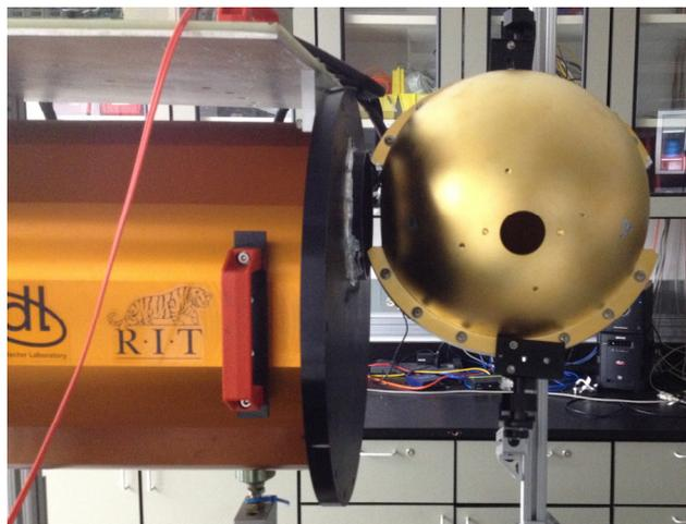
*Figure 26. This image shows a gold-coated integrating sphere attached to one of the dewars. The gold coating is more reflective in the infrared than the more commonly-used integrating sphere that is coated with white paint that is highly reflective at optical wavelengths.*
