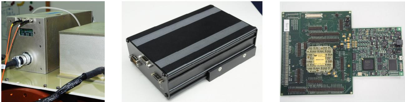
Figure 18. The three electronics packages used to test detectors. Electronics from left to right: Astronomical Research Camera Controller; JMClarke Engineering, Teledyne SIDECAR ASIC.
