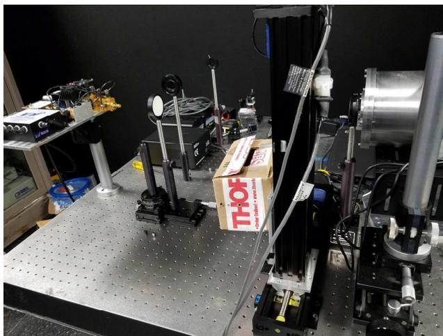
Figure 18. A photo of experimental THz scanner setup is shown above. The source is on the left, followed by the Teflon lens, and the test dewar enclosure on the right. The thor lab box, containing various targets, is mounted on XYZ and rotation stages for scanning.
