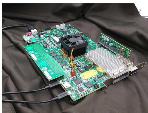
Figure 32. Shown above is the Xilinx FPGA used to create the PEK Evaluation Test Bed.
