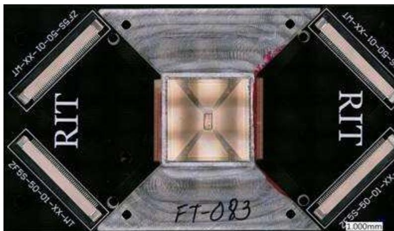
Figure 12. The photo above shows a packaged integrated photonic chip connected to printed circuit boards integrated into an RIT testbed.
