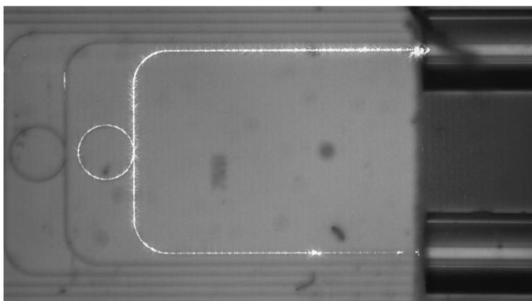
*Figure 25. In the picture, you can see fiber coupling to the integrated aluminum nitride waveguides and microring resonators. A frequency doubled continuous wave Ti:Sapphire generating 369 nm is fiber coupled and that fiber is edge coupled to the aluminum nitride waveguide. A second fiber collects the residual pump light and any new frequencies generated via nonlinear processes in the integrated circuit at the output port to where it is sent various pieces of measurement equipment.*
