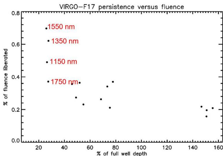
Figure 7. This figure shows the persistence vs fluence plot for F17 at 1150, 1350, 1550, and 1750 nm.
