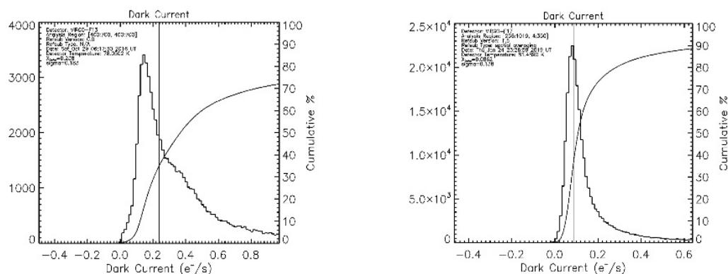
Figure 6. This figure shows the dark current histograms for detectors F13 (left) and F17 (right) at 80 K.
