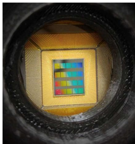
Figure 26. This picture shows twenty 1 Mpixel QIS arrays residing in the detector housing.
