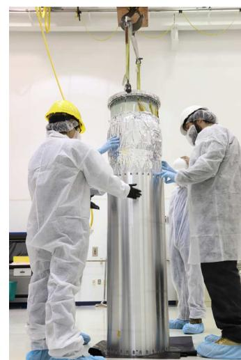
*Figure 14. Chi Nguyen and her collaborators are lifting the experiment out of the rocket skin in the clean room at Wallops Flight Facility.*
