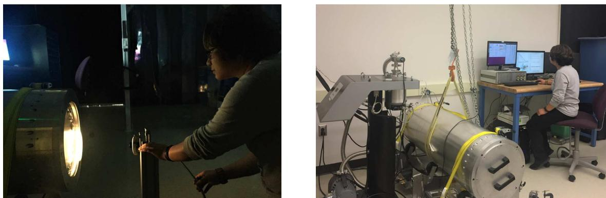
*Figure 57. (left) In the picture above, Chi Nguyen measures light levels while characterizing the CIBER-2 payload. (right) Nguyen monitors the temperature for CIBER-2 during an experiment in the Suborbital Astrophysics Lab.*
