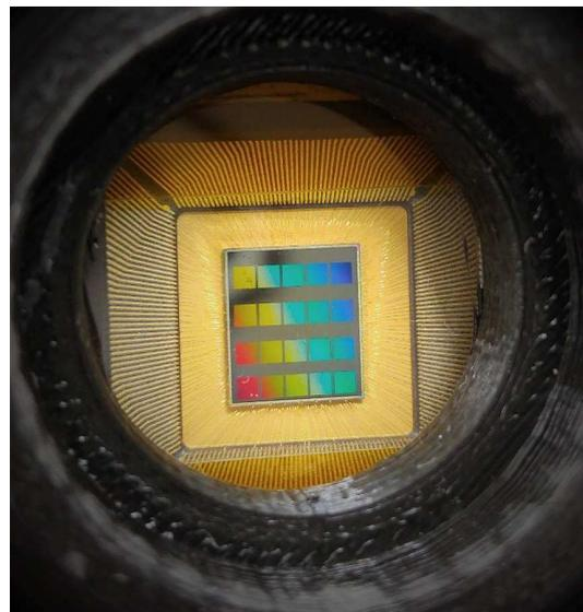
Figure 3. The image above shows twenty megapixel QIS arrays residing in the detector housing. Each detector has a side length of  $1.1 \mu\text{m}$ . All twenty detectors fit within a square millimeter.
