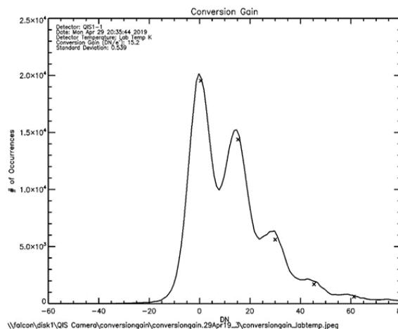
Figure 4. The graph shows the distribution of signal in the conversion gain analysis. The location of peaks corresponds to integer numbers of electrons detected as a signal. Location of peaks is determined from gaussian fitting and subtracting.
