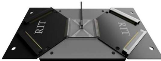
*Figure 35. Shown above is a CAD rendered image of the prototype packaging solution currently in development, allowing for optical and electrical interconnects in a confined space. The PIC chip is bonded to an interposer (fabricated in the RIT SMFL) and then routed to two PCB boards; a fiber array provides the optical interconnect.*
