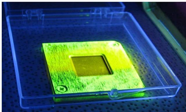
*Figure 20. The yellow/green device above is a Quantum Dot coated detector in aluminum mask under UV illumination. The active area is 15 mm×15 mm.*
