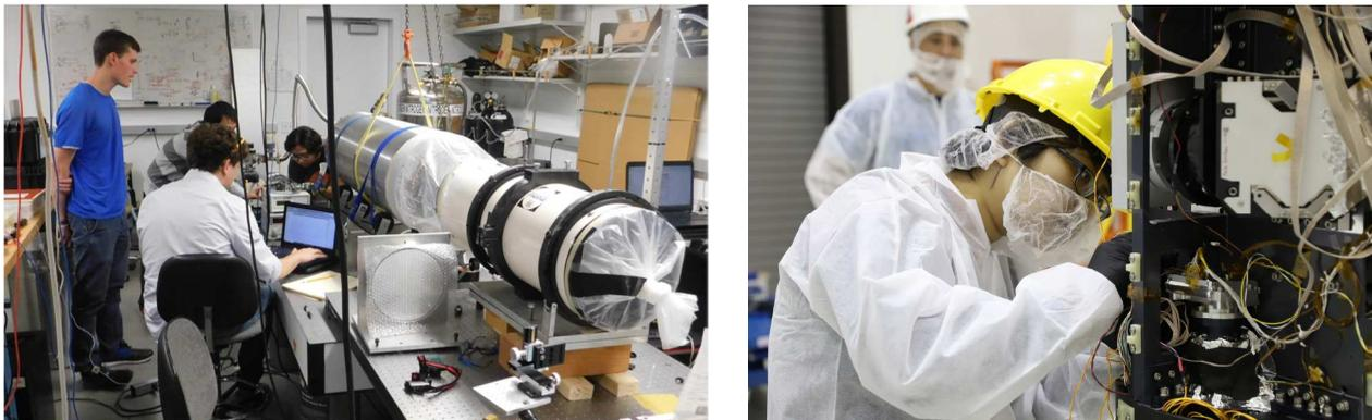
*Figure 11. (left) CfD students monitor the CSTARS-2 detector as it captures images at a cryogenic temperature inside the CIBER-2 rocket skin at Caltech. (right) Chi Nguyen checks the CSTARS-2 mechanical components before the payload undergoes environmental testing at the Wallops Flight Facility.*
