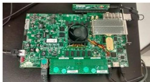
Figure 24. Above is the Xilinx VCU108 FPGA board that Davis used as the programmable system for communication between the user interface and peripheral QSFP modules.
