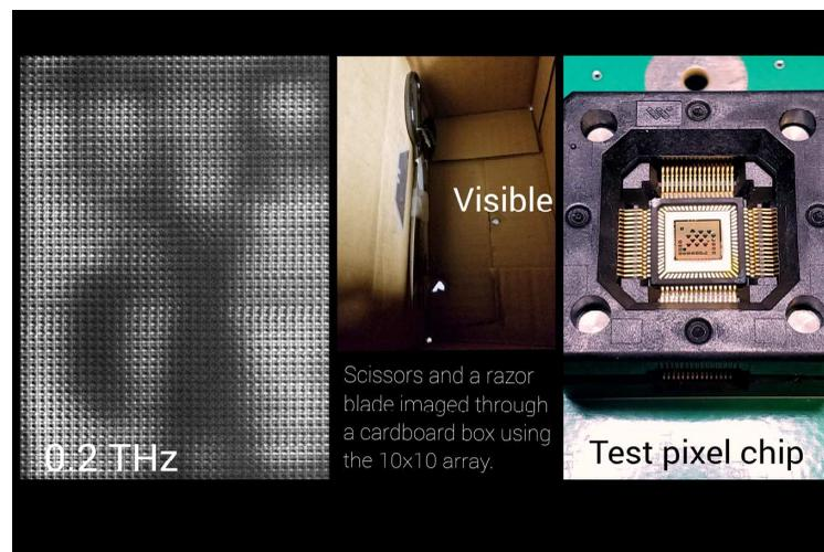
Figure 33. (left): A 0.2 THz mosaic image of the scissor and razor blade enclosed in a box as imaged by the 10x10 pixel array is shown. The pattern visible is due to variations of pixel response and will be accounted for using the power relation found from work with single pixel testing. (middle): You can see a visible image of the inside of the box. (right): Pictured here is a close up of one of the single pixel chips with varied designs.
