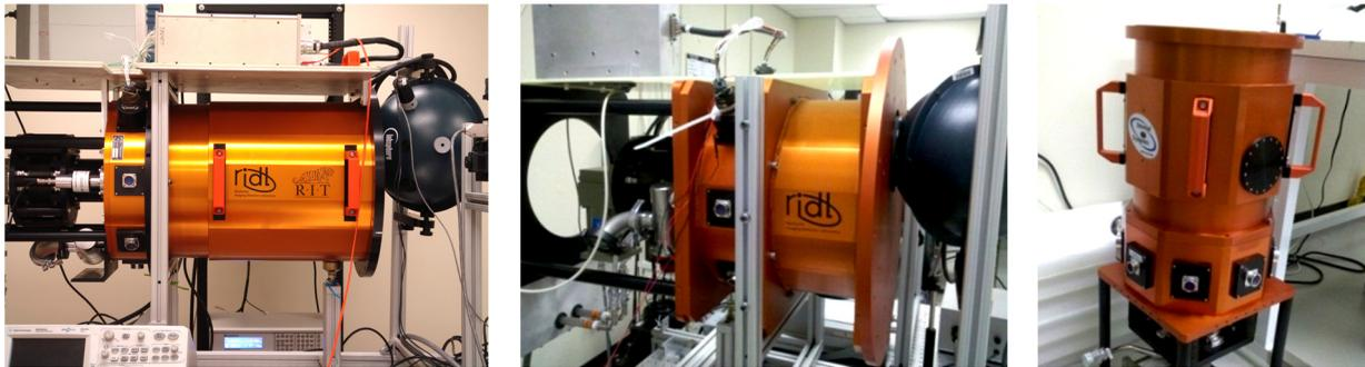
Figure 53. Detectors are evaluated in four custom dewar test systems. The fourth dewar (not pictured) is a duplicate of the one on the left.
