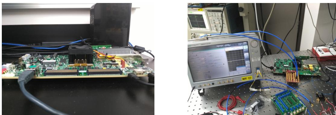
Figure 39. (left) The picture shows the initial setup of the VCU108 FPGA. (right) The image shows the FPGA connected to a RF analyzer.
