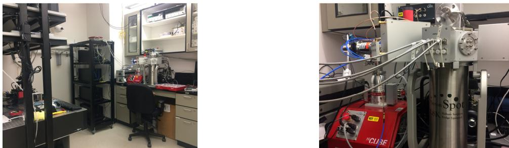
Figure 56. (left) The Integrated Photonics Group acquired space to create the Integrated Photonics Lab to run quantum integrated photonic experiments. (right) Located in the lab is a Photon Spot single photon detector system funded by AFOSR.
