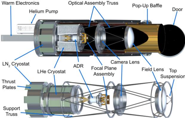
Figure 33. The image above is a mechanical model for a NASA proposed project, the Rocket Axion Decay Experiment (RAXDEX)
