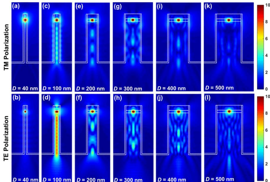
Figure 14. (top) This shows the cross-sectional near-field electric field intensity of nanowire UV LEDs with  $H = 1 \mu\text{m}$  and various diameters for TM-polarization (bottom) and TE-polarization.
