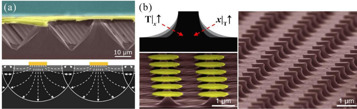
Figure 35. (left) This image shows the fabrication of suspended III-V nanofoils by inverse metal-assisted chemical etching of  $\text{In}_{0.49}\text{Ga}_{0.51}\text{P}/\text{GaAs}$  heteroepitaxial films, and (middle) ordered  $\text{Al}_x\text{Ga}_{1-x}\text{As}$  nanopillar arrays via inverse metal-assisted chemical etching.
