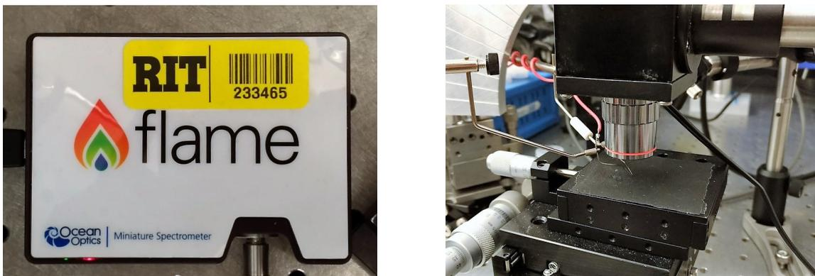
Figure 58. The electroluminescence measurement setup includes a rotating testing stage (right) and a FLAME 200 nm – 850 nm spectrometer (left).
