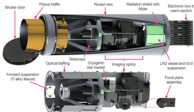
Figure 16. Seen above is a solid model of the CIBER-2 Payload. All components are being integrated and validated.
