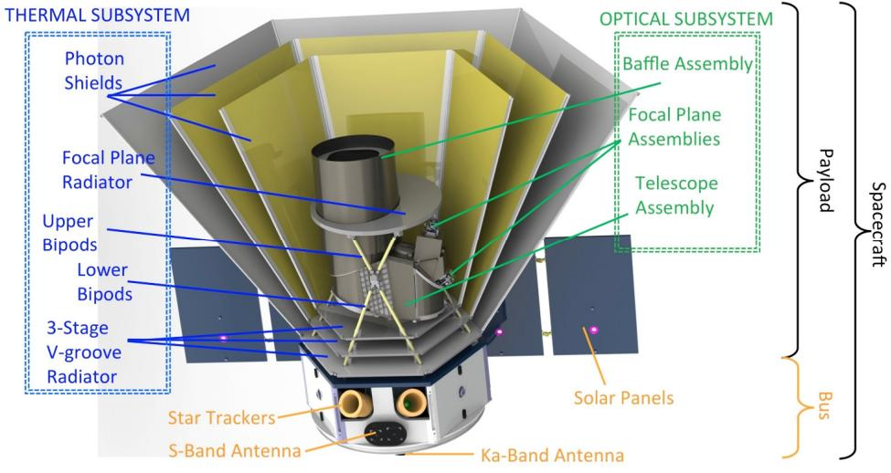
Figure 47. The image shows the design of SPHEREx. Credit: NASA.
