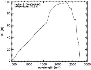
Figure 2. The QE of a thinned part extends below 1.1 μm, as expected.
