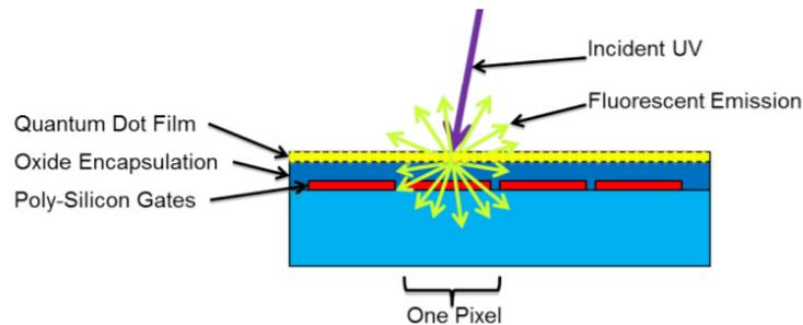
Figure 29. The cross-section schematic shows a quantum dot coated device.
