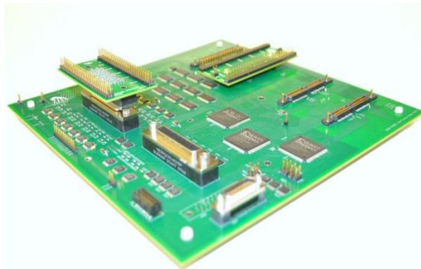
*Figure 63. This image shows a cryogenic multi-layer circuit board designed in the CfD and populated in CEMA. All of the components on this board work at temperatures as low as 40 K, nanoTorr pressure levels, and in the presence of high energy particle radiation.*
