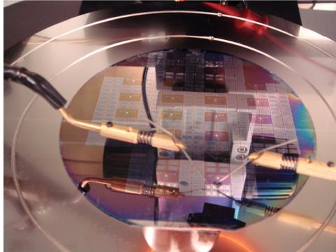
*Figure 62. This image is a close-up of a device wafer being tested on the probe station.*
