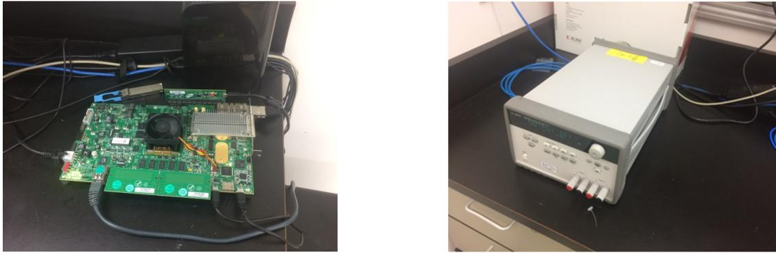
Figure 40. (left) Show in the photo is a VCU108 FPGA board made by Xilinx used in the EVT system. (right) The Agilnet E3649A power supply is being used in testing ProberControl.
