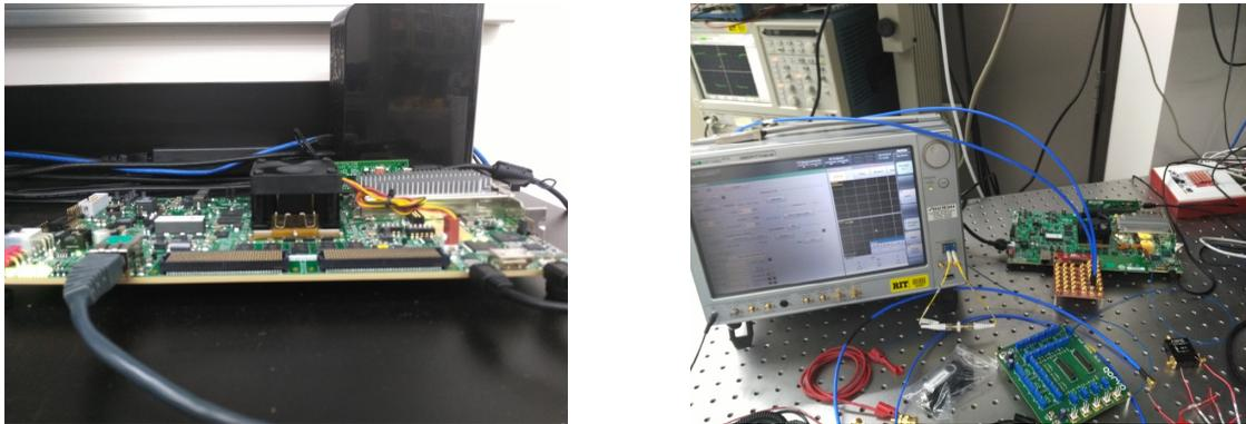
Figure 39. (left) The picture shows the initial setup of the VCU108 FPGA. (right) The image shows the FPGA connected to a RF analyzer.
