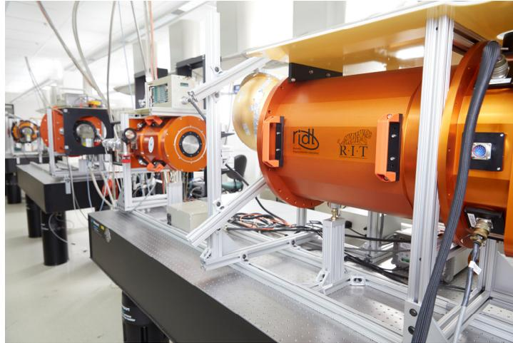
*Figure 51. The photo shows cryogenic dewars in the Rochester Imaging Detector Laboratory.*
