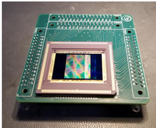
Figure 11. (left) Undergraduate students Ben Stewart and Ambar deStantiago complete telemetry stream interfacing at the NASA Wallops Flight Facility. (right) The project used a 5.5 megapixel sCMOS detector mounted on a custom printed circuit board.
