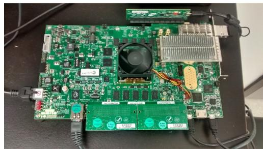
Figure 37. (left) A Xilinx VCU108 FPGA will be used in the EVT station to host various devices, such as a QSFP based package developed by Precision Optical Transceivers (right).
