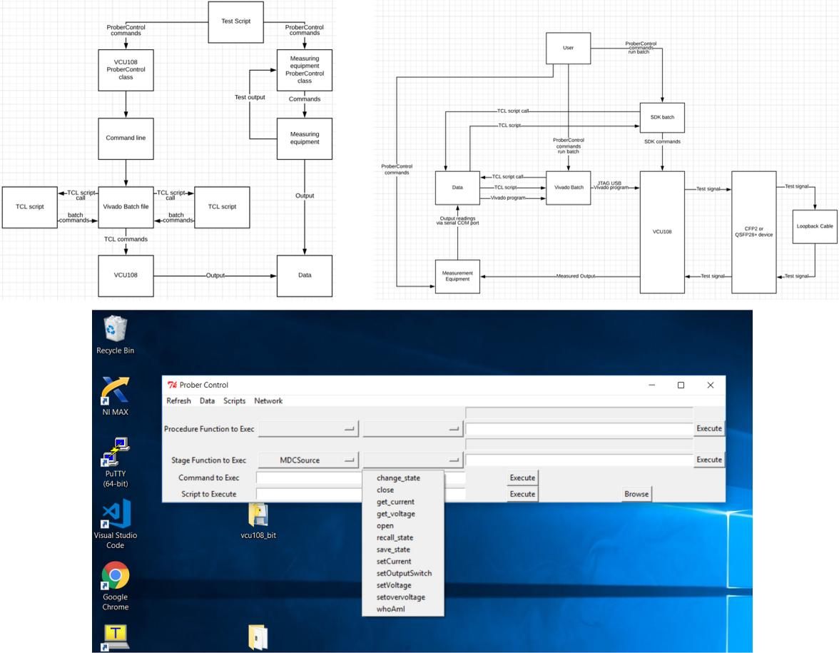
Figure 19. The charts show draft versions of the software flow (top, left) and communication flow (top, right) diagrams for the EVT project. The Prober Control software program (bottom) is the executive processor for scripts used in the EVT.
