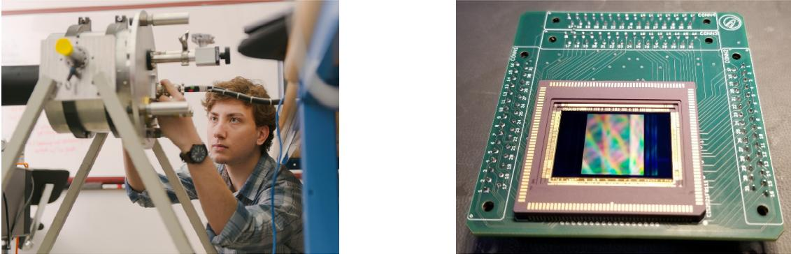
Figure 32. (left) Ben Stewart works on the creation of the cryogenic star tracking attitude regulation system. (right) Shown here is a sCMOS detector mounted to focal plane printed circuit board.
