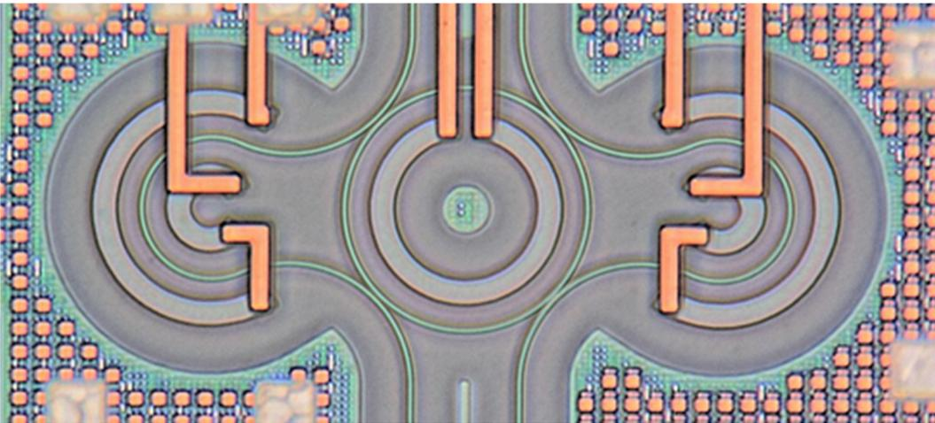
Figure 6. Above is a microscope image of an entangled photon source on an integrated photonic chip.
