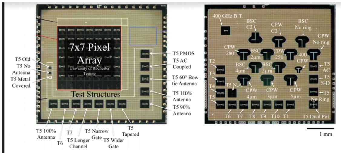
Figure 34. The above devices were designed locally for the THz imaging project.
