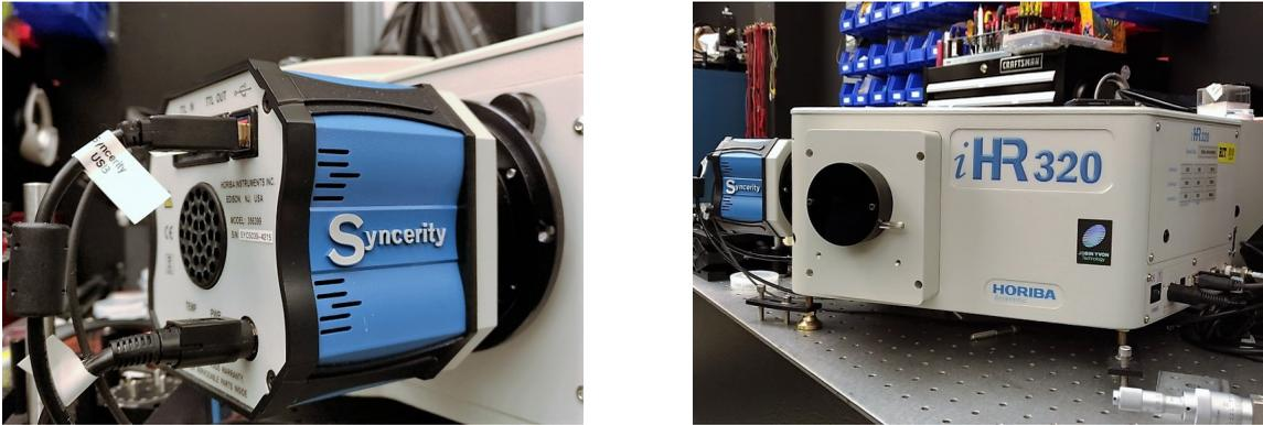
Figure 57. The Sincerity CCD Array detector (left) and the HR320 spectrometer (right) are part of the photoluminescence system.
