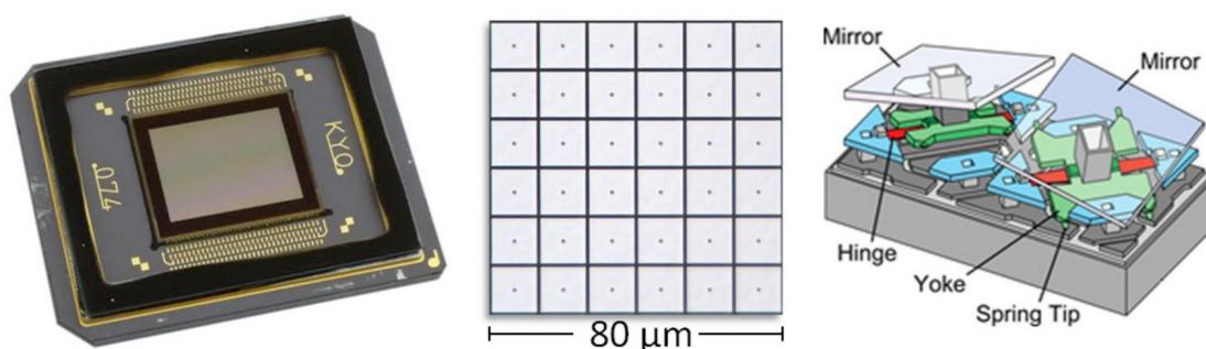
Figure 22. (left) The picture shows a DMD with a custom UV-enhanced sapphire window. (middle) A microscope image shows 36 individual micromirrors. (right) A schematic shows the hinge and tilt mechanism for two micromirrors.
