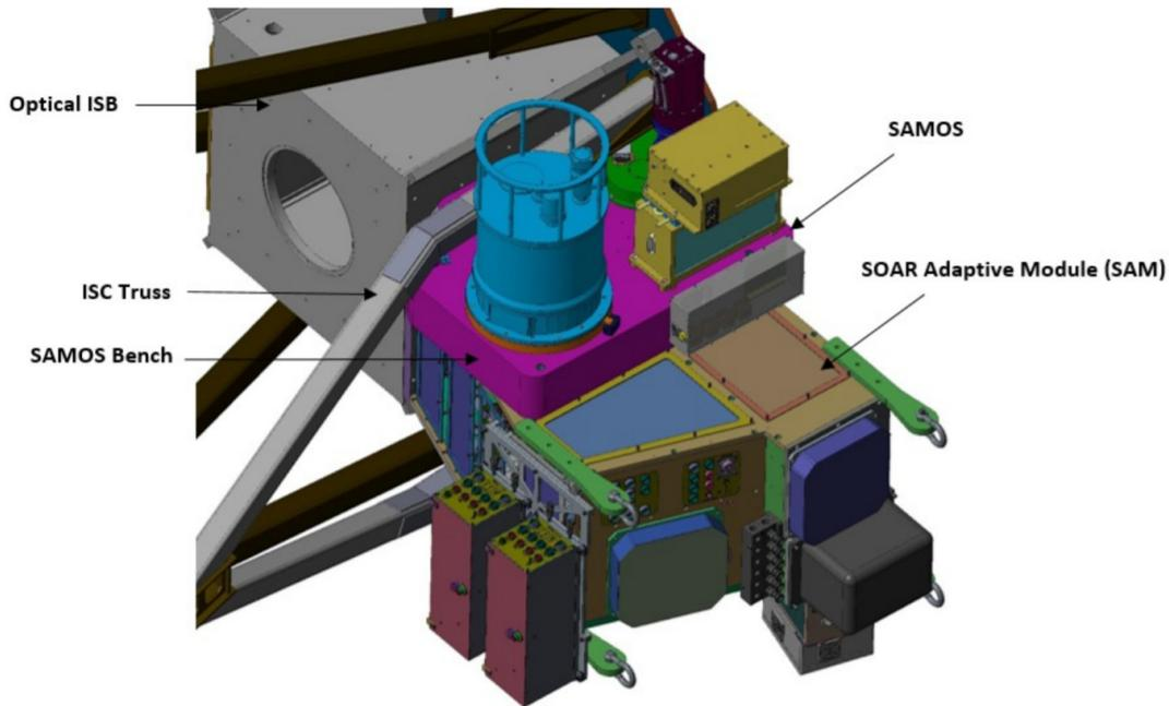
Figure 28. In the rendered image, the SAMOS is mounted to the SOAR Adaptive Module.
