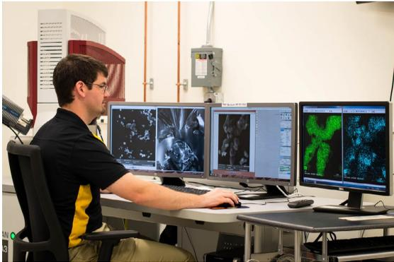
Figure 65. (left) PhD student Mohad Baboli loads a sample in the AIXTRON 3x2 Close Coupled Showerhead metal-organic chemical vapor deposition reactor, part of the MOVPE. (right) PhD student Thomas Wilhelm uses a TESCAN MIRA3 scanning electron microscope to analyze samples for use in metal-assisted chemical etching experiments.
