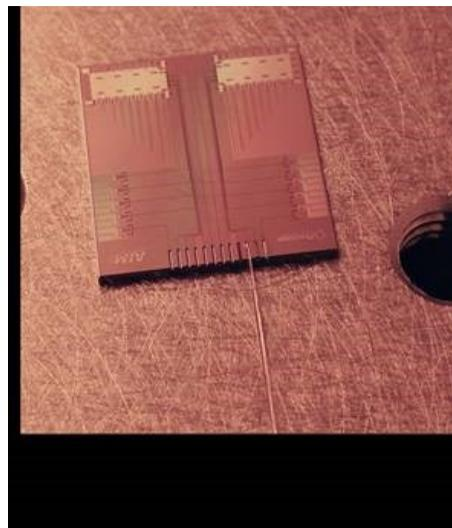
*Figure 12. This integrated photonic chip, designed by Precision Optical Transceivers and fabricated by AIM Photonics uses an optical fiber for input and output.*
