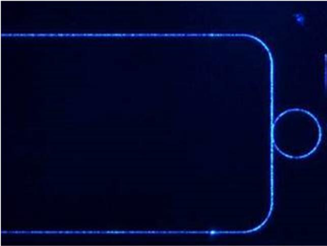
Figure 5. The image shows visible light propagating in an aluminum nitride waveguide and ring resonator.
