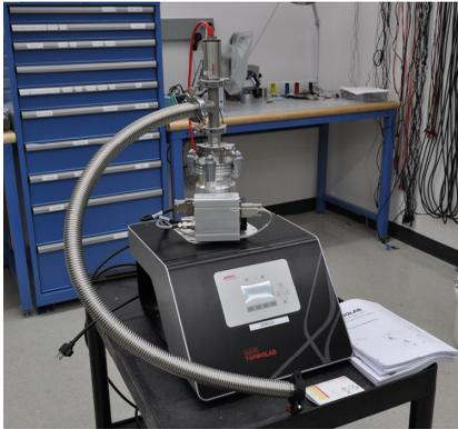
Figure 64. (left) Pictured here are the function generators, oscilloscopes, and FPGA-based control boards used to develop an image sensor readout package that will fly on a suborbital platform. (right) The picture shows one of the Oerlikon Leybold Turbolab turbo-molecular pumping stations in the lab.
