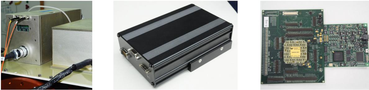
Figure 52. The three electronics packages used to test detectors are the Astronomical Research Camera Controller (left), JMClarke Engineering (middle), and the Teledyne SIDECAR ASIC (right).
