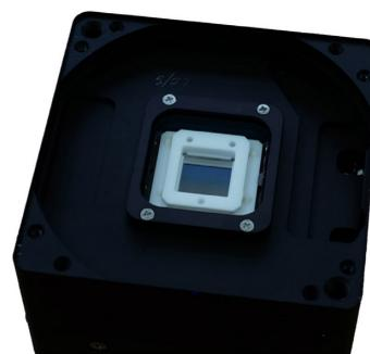
Figure 20. RITPIC uses a CCD and a MOXTEK, Inc. micropolarizer array. Shown above, the micropolarizer array (silver square) is aligned and affixed to the CCD using a white ceramic carrier. The polarization-sensitive imager is inside a camera body, allowing thermoelectric cooling.
